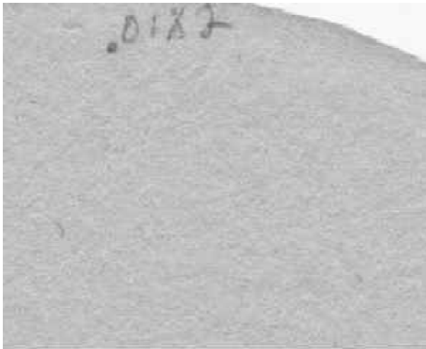
Figure 2: Magnified section of the dry 0.01 % wax on OCC in virgin kraft, 2.4 gm hadsheet including the label mark at the top center. There is no evidence of wax.
